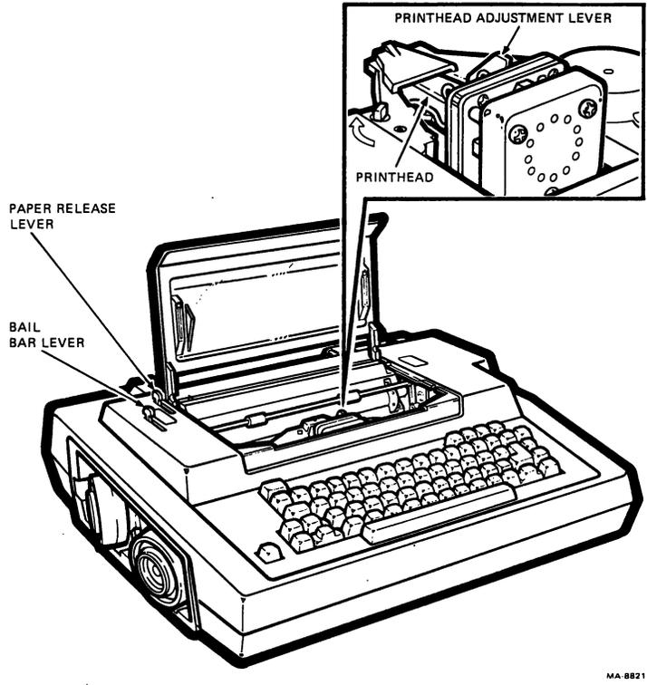
Figure 1-3 Printer Control Levers
