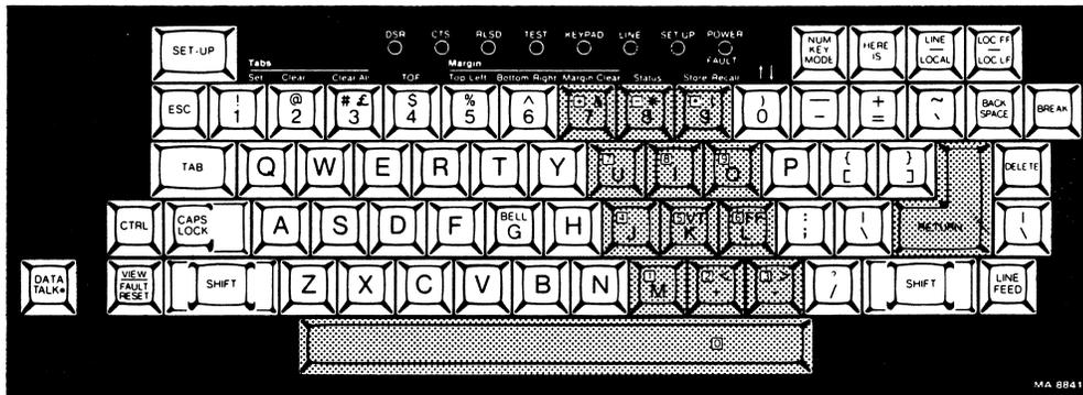
Figure 1-5 Standard Keyboard with Imbedded Keypad
