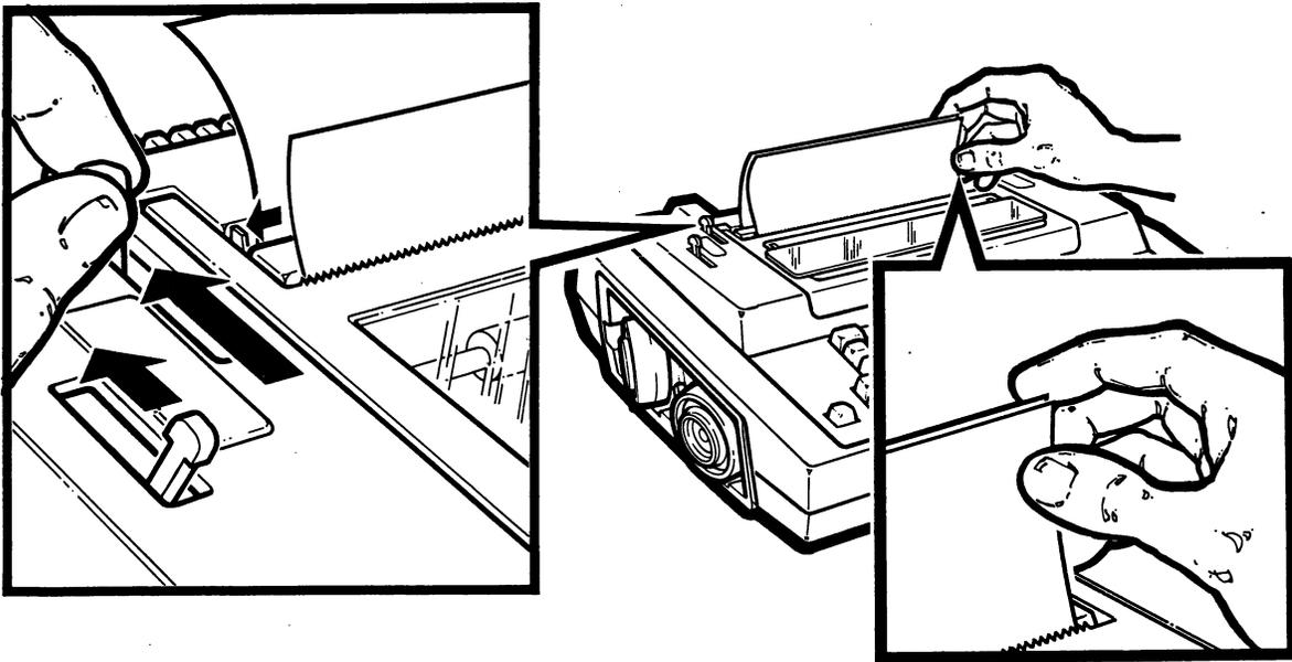
Figure 2-3 Loading Single Sheet Paper (Sheet 2 of 3)
