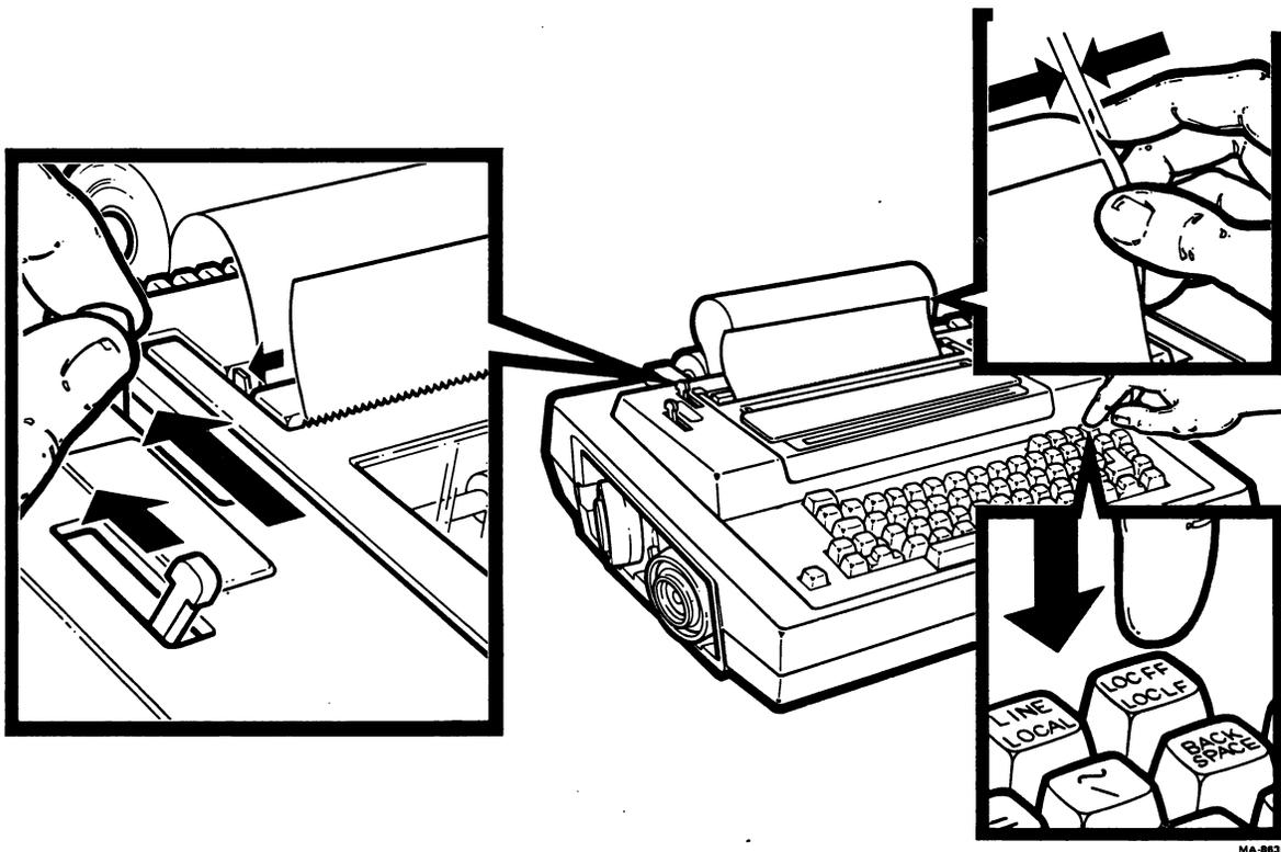
Figure 2-5 Loading Roll Paper (Sheet 2 of 3)
